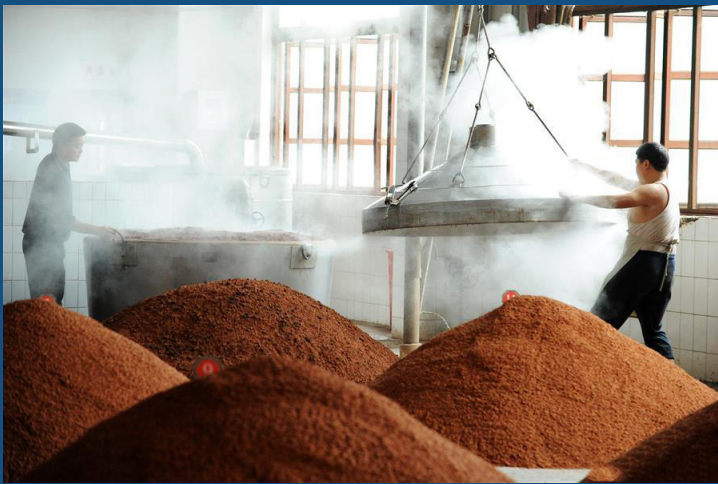
Image: Gafencu, Workers mix grains with yeast
